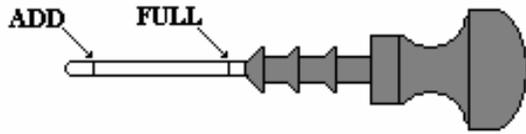
1. Maintain the engine oil level between “ADD” mark and “FULL” mark on Oil Level Gauge. Do not fill crankcase above “FULL” mark.
